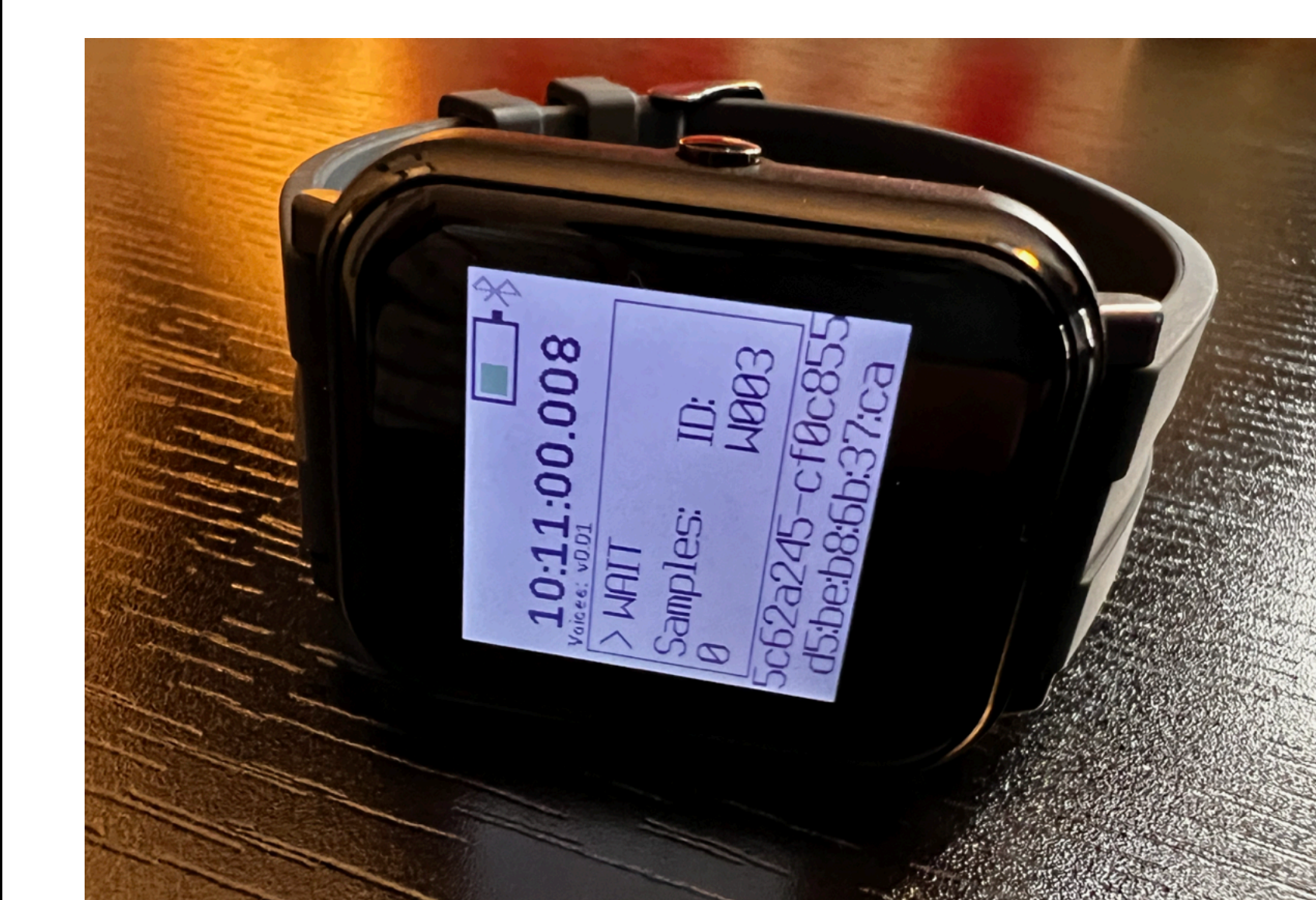
Figure 2. Bangle.js 2 watch running the BEATwatch application. Watches are easily attached to participants' wrists, record PPG data to internal storage, and transfer completed records via BLE.
